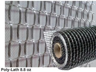
3D is a Leno Style weaved tightly twisted yarns to create a three dimensional, self-furring, open weave glass fibered lath. 1/4" Thick Poly-Glass fiber reinforcement lath is designed for use with traditional wall systems and cement applications. Self-Furring, Alkali Resist Lightweight, 31 lbs. per roll. Omni-directional, can be rolled out horizontally or vertically. Suggested Fasteners: 1-3/4" Anchor Plate with appropriate screw fastener
